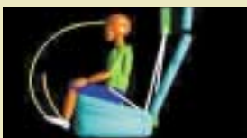
6 year-old child dummy, restrained by only the lap belt. 35 mph frontal crash. Extensive dummy movement.
