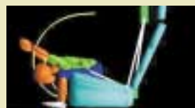
6 year-old child dummy, restrained by only the lap belt. 35 mph frontal crash. Extensive dummy movement.
