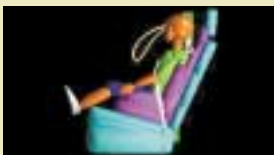
6 year-old child dummy in a belt-positioning booster seat, restrained by a lap-shoulder belt. 35 mph frontal crash. Little dummy movement.
