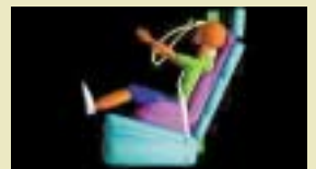
6 year-old child dummy in a belt-positioning booster seat, restrained by a lap-shoulder belt. 35 mph frontal crash. Little dummy movement.
