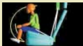
6 year-old child dummy, restrained by only the lap belt. 35 mph frontal crash. Extensive dummy movement.
