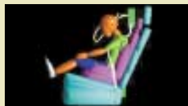
6 year-old child dummy in a belt-positioning booster seat, restrained by a lap-shoulder belt. 35 mph frontal crash. Little dummy movement.
