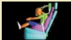
6 year-old child dummy in a belt-positioning booster seat, restrained by a lap-shoulder belt. 35 mph frontal crash. Little dummy movement.
